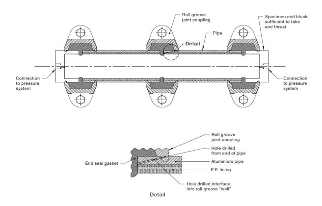
FIGURE C1 TYPICAL TEST APPARATUS
